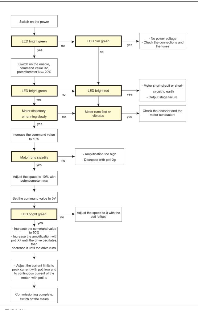
Functional diagram bl/ec motor amplifier
