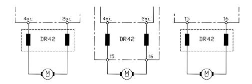
The motor lines are only allowed to be switched when the mains current is disabled. Any switching-off when connected to current will cause arcing. Any switching-on when the controller is enabled may damage the motor.
