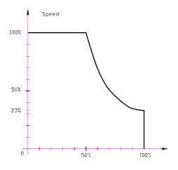
Take this motor curve as an example. The linear limit characteristic of the servo-amplifier must be within the motor characteristic.
