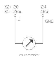
The command value input can be switched as a differential input or as an input amplifier with reference to point zero, depending on how the switch S2:K2 is switched.
