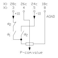
Input X1:26c (X1:4) command value Input X1:18c (X1:8) command value Voltage X1:26c - X1:18c 0 to  $\pm$  10V Input resistance 50 k $\Omega$
