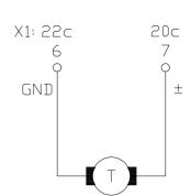
For armature voltage control with IxR compensation the armature voltage  $U_A$  is internally connected by means of the switch S6:K4.
