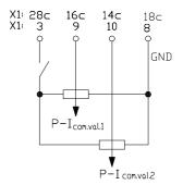
Input X1:16c (X1:9) current limiting I1, 0 to +10V
