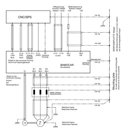
The units comply with the EC Directive 2004/108/EC in the standards EN61800-3 under the following installation and test conditions
