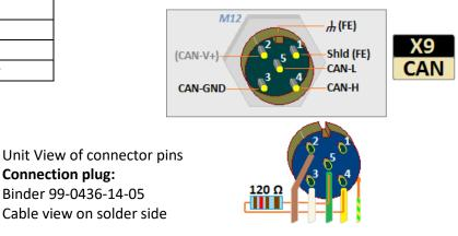
Termination resistor at both ends of the bus line / 120 Ohm between CAN-H and CAN-L
