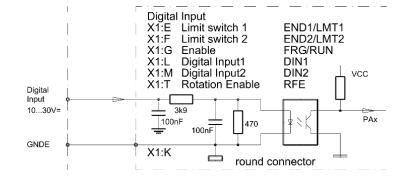
The enable input (FRG/RUN) and the input for rotating field enable (RFE) are permanently assigned and cannot be programmed.
