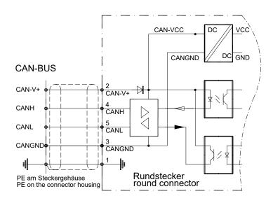
The BUS interface is galvanically separated from the internal device voltage.
