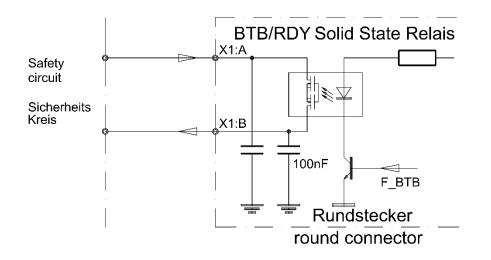
Contact for max. 48 V / 0.5 A (not short-circuit-proof) Capacitive load: max. 1  $\mu$ F Contact resistance: max. 2  $\Omega$
