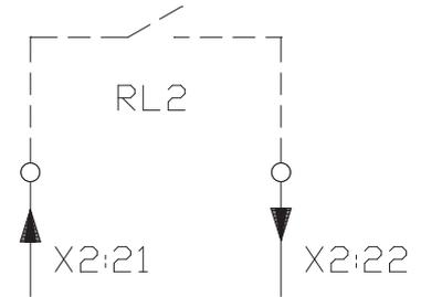
The BTB contact signals to the PLC/CNC that the drive is functional.
