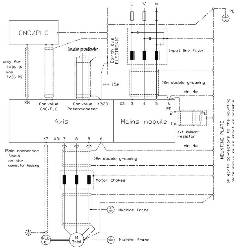
The devices adhere to the EU guidelines 89/336/EWG and the technical standards EN 610001-2 and 61000-4 provided that the following conditions are observed:
