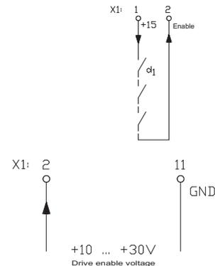
**Drive enable - external logic voltage**
