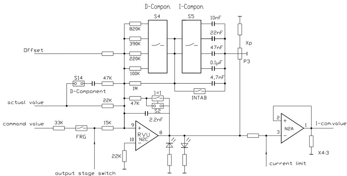
Adjustment of the proportional term by means of the binary switch S4
